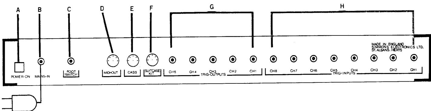
Looking at the back of TMI you will see on the extreme left hand side is the 'POWER ON/OFF' switch (A). The unit is powered up with the switch in the down position. To the right of that is the power connector (B). Connect this to your domestic mains supply – make sure you have the correct voltage TMI.
