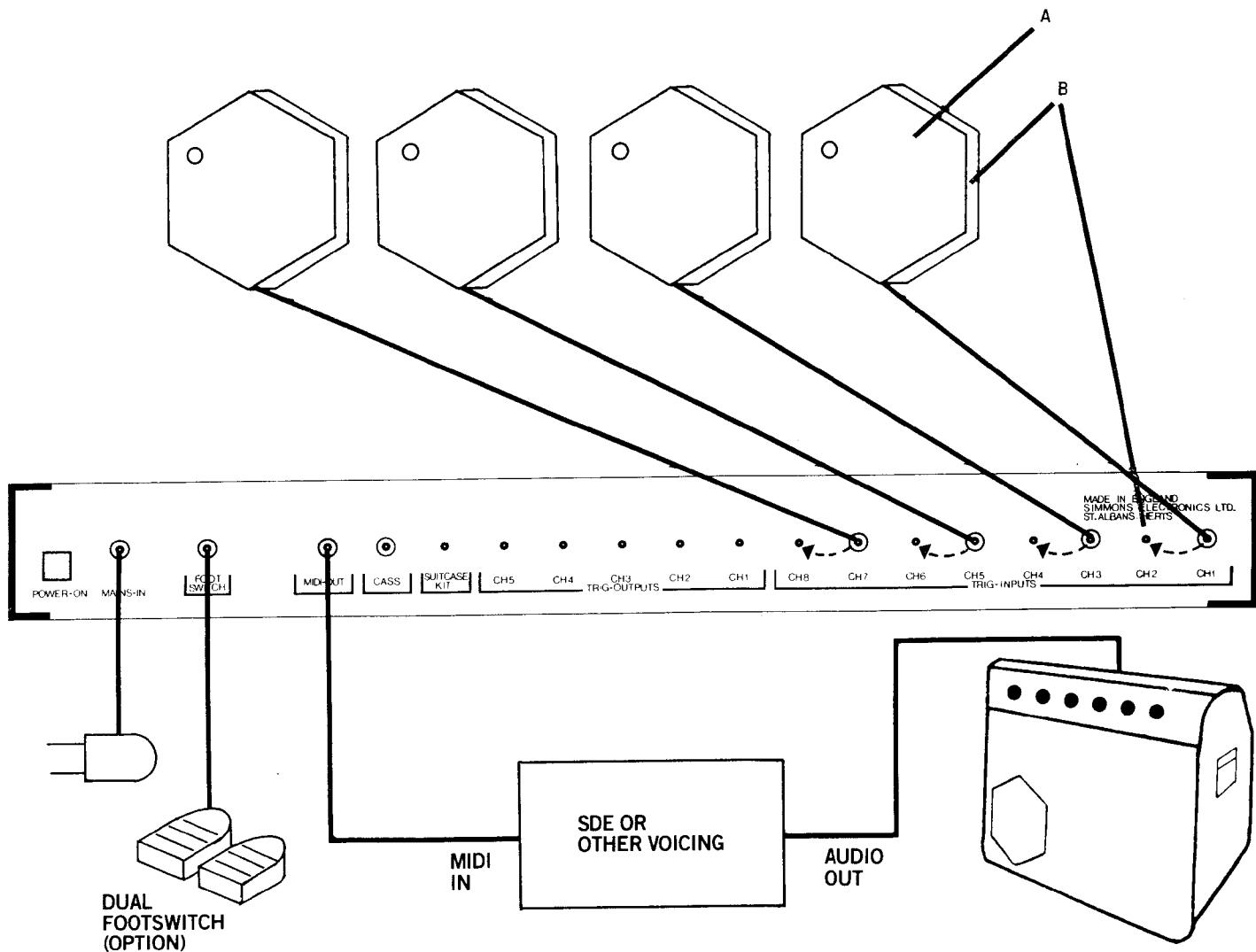
Simmons' stereo pads can be used to play different sounds on the playing surface (A) and the rim of the pad (B). In this case each stereo pad uses two channels on TMI. Channels 1, 3, 5 and 7 are wired in such a way that if you insert a stereo jack plug into these sockets channels 2, 4, 6 and 8 are routed respectively to the rims on the stereo pads.
