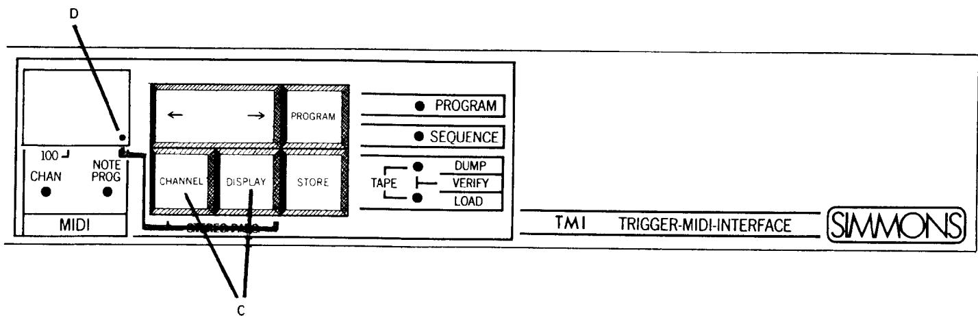
You have to switch TMI to a special 'STEREO PAD MODE' which eliminates 'cross talk' from the pads.
