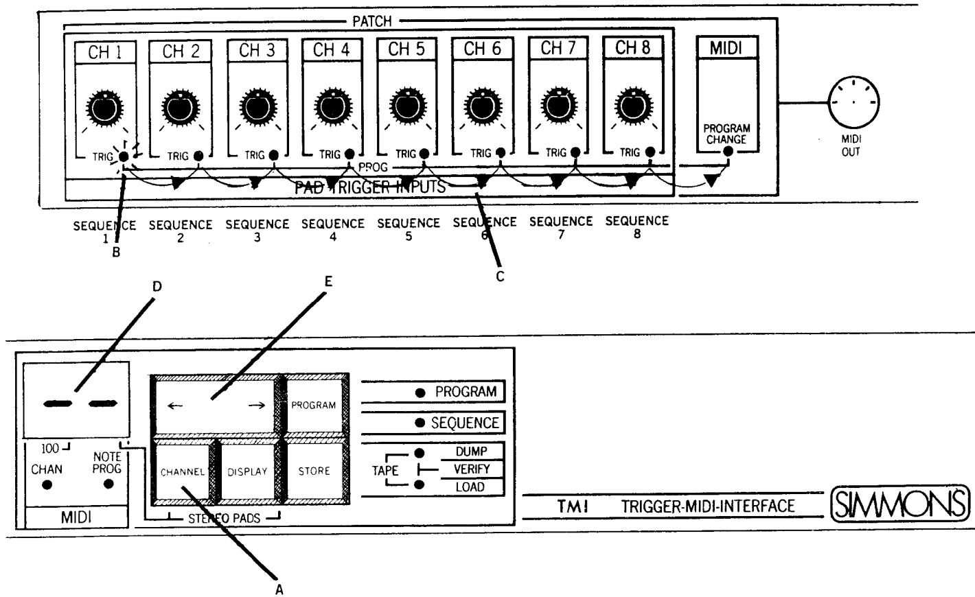
Whilst you are in playback mode press 'CHANNEL' (A). You will see that channel 1 trigger LED lights up (B). In this 'playback sequence' mode the 8 channel trigger LEDs take on the function of displaying the sequence number that you are playing back (if a channel is triggered when the LED is used for playback sequence then it will flash 'off - on' rather than 'on - off').
