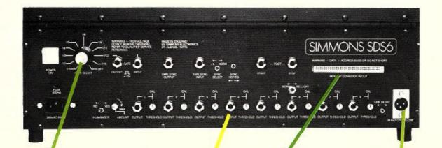
Comprehensive sync inputs and outputs allow the SDS 6 to work with a multitude of electronic equipment. The expansion buss allows the SDS 6 direct access to external memory packs, which it can read in less than half a second.
