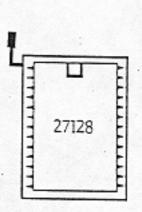
WARNING MAKE SURE THE SAFE/BLOW SWITCH IS SWITCHED TO SAFE BEFORE INSERTING OR REMOVING EPROMS OTHERWISE YOUR SAMPLES WILL GO 'CRUNCHY'!
