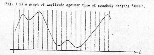
The amplitude of the signal can be represented by a number and if the wave form is measured at regular intervals these numbers would represent the change in amplitude of the signal over time.
