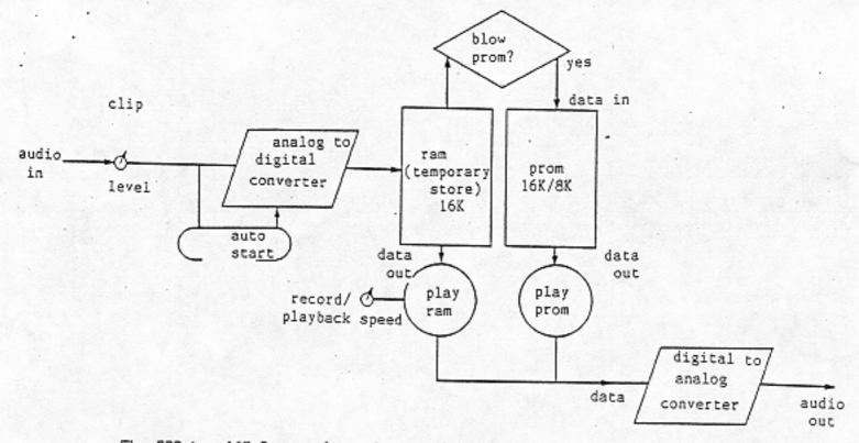
The EPB has 16K Bytes of sample ram which is used when a sound is sampled. This ram is arranged in 2 x 8K blocks. So that if you wish to sample a short sound you can switch to 8K and save on the cost of proms. (8K proms being approx half the price of 16K proms).
